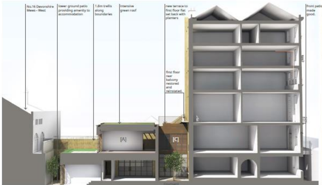
Sectional view showing the proposed extension
